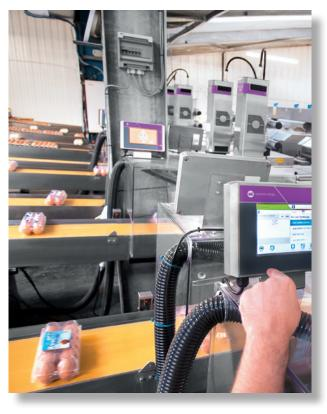
An intuitive touchscreen makes SmartLase C350 easy to use and helps to reduce operator errors.
