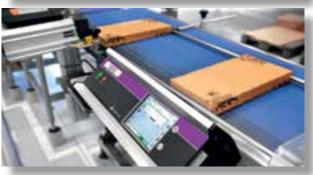
To code packaging film Hotel Chocolat installed two SmartDate coders on each of its production lines. Shipping boxes are coded with a high resolution hot melt inkjet printer.
