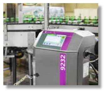
At HEINEKEN, in Marseille, nine 9232 printers were installed on the various production lines (bottles and packs).
