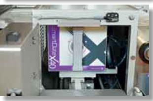
At Saint-Jean, the installation of SmartDate X40 thermal transfer coders has been optimized: the printhead is protected and is placed at operator height to make life easier for production line operators.
