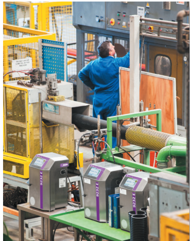
Fifteen 9232 E inkjet printers using white ink code Polypipe's extruded pipe work.
