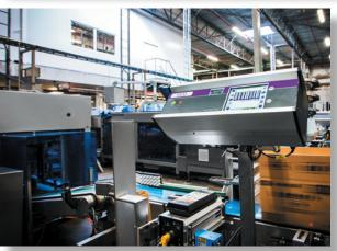
With the 5800 coders, Farm Frites could replace its pre-printed cartons by blank cartons personalized at the last moment.
