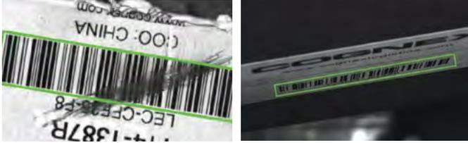
**1DMax® with Hotbars®** is optimized for omnidirectional 1D barcode reading and decodes low-resolution codes up to 10X the speed of a conventional barcode reader.
