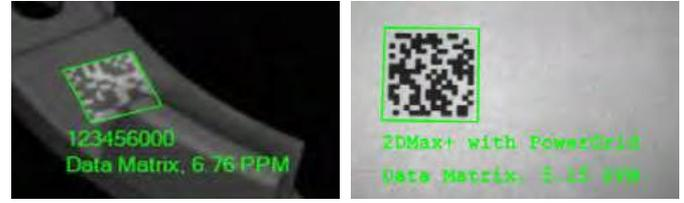
**2DMax® with PowerGrid®** is designed to read 2D codes with significant damage or complete elimination of finder and clocking pattern, or quiet zone.
