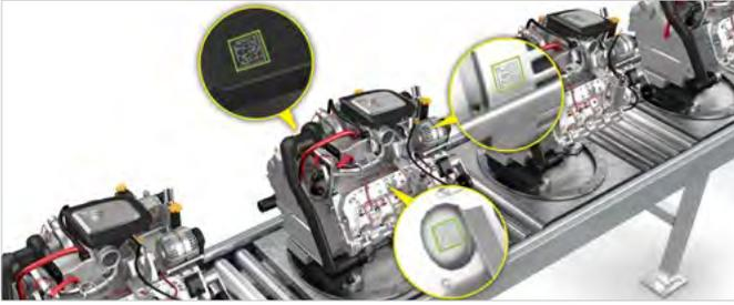
Integrated **diffuse, polarized, and direct lighting** enables superior image formation to read dot peen, laser-etched, and label-based codes on challenging (shiny, cylindrical, dark) surfaces without any hot spots.
