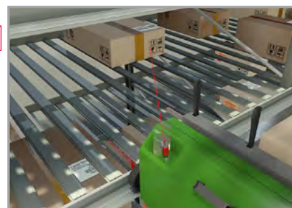
Multi-depth compartment occupation check
