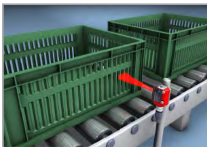
XL Spot - Detection of slotted objects
